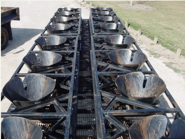
Top view of the tree transport trailer, developed by the City of Wichita Falls to increase staff productivity and efficiency.
